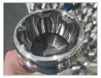
Workpiece: CV joint Workpiece material: S55C Workpiece hardness: HRC58-62 Machining position: Inner diameter Machining type: Interrupted finishing
