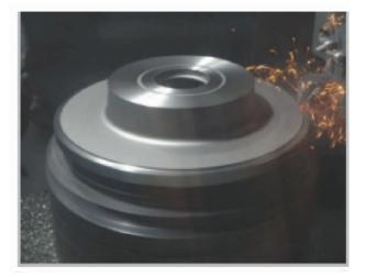
Workpiece: Brake disc Funik CBN cutting tool: The life is increased by The efficiency is promoted by Workpiece material: GG25 Workpiece hardness: HB190-210 Machining position: Brake surface
